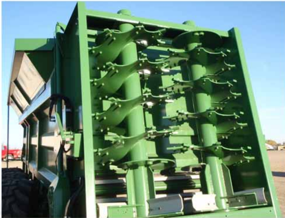
Vertical Auger spreader
