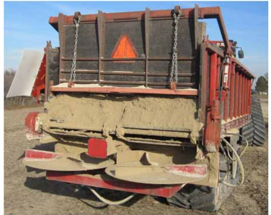
Twin spinning disk broadcast spreader
